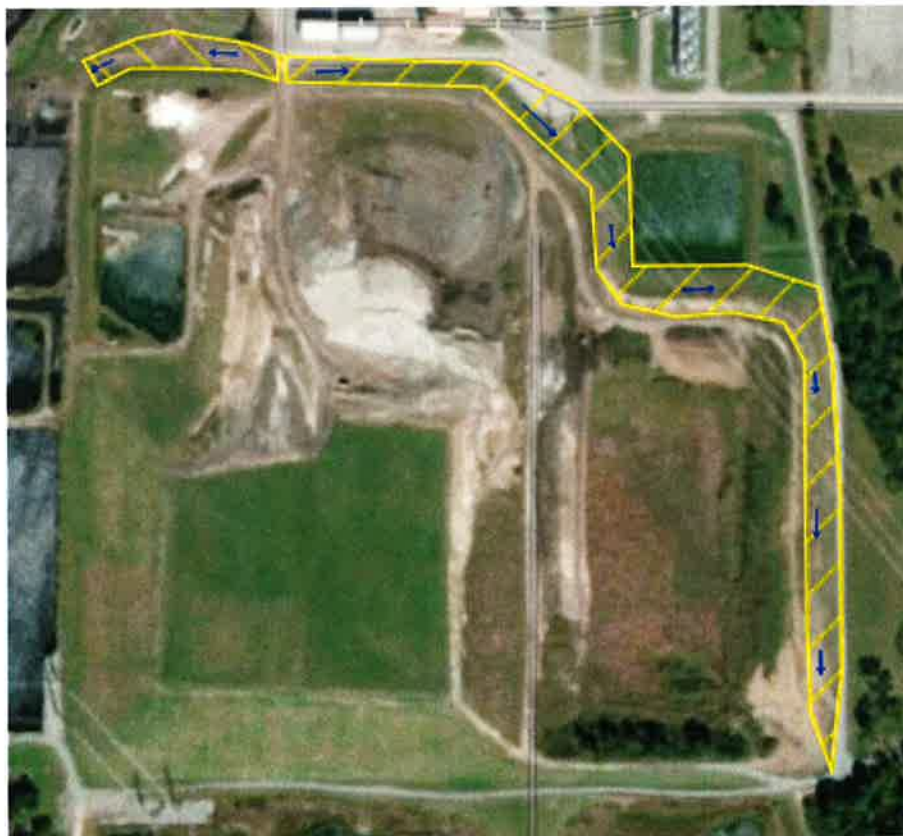
Figure 3-1 Run-On Areas and Drainage Direction
