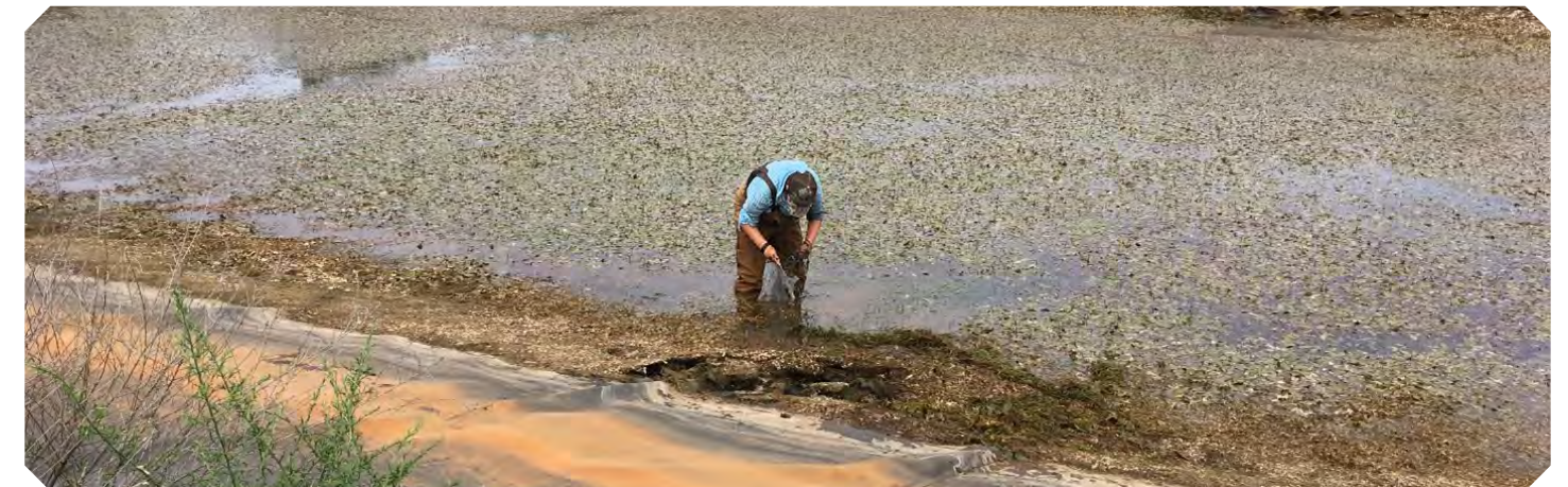
Sampling substrates from one of the vertical flow bioreactors at the Mayer Ranch passive treatments system near Tar Creek.
