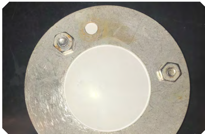
A Polar Organic Chemical Integrative Sampler
