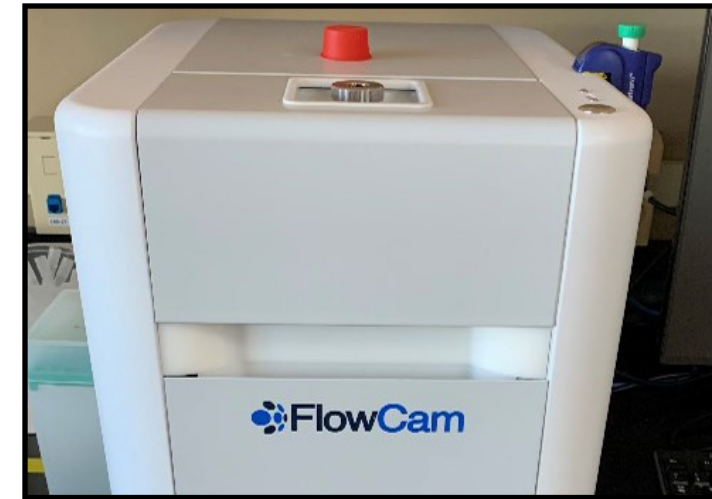
Figure 9: GRDA's Flowcam used to identify & quantify algae
