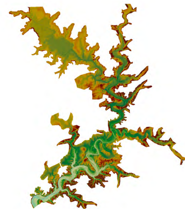
Image of a TIN model for the full study area with bathymetry
