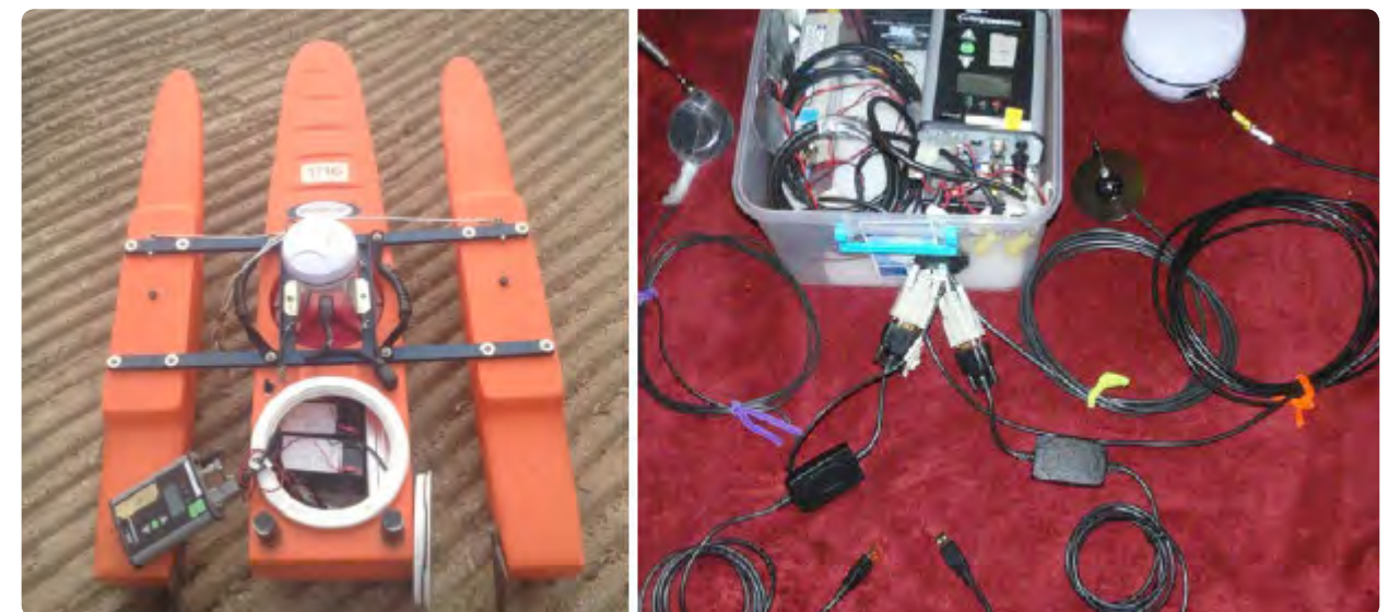
Acoustic Doppler Current Profiler (ADCP) setup showing a trimarian (left) and a base station (right)
