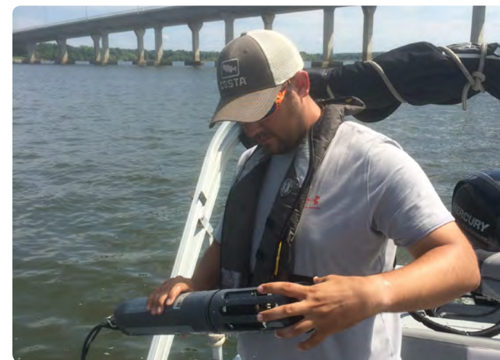
Dustin Browning - GRDA operates a water quality sonde
