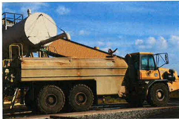
Figure 4.7 Typical Water Truck for Fugitive Dust Control John Deere Model 300D; 7,000 gallon capacity (or comparable)
