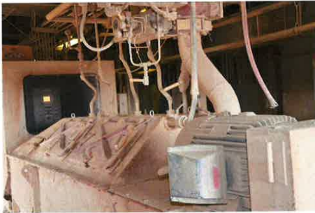
Figure 4.2 Pin & Paddle Mixer (Preparation of Conditioned CCR)
