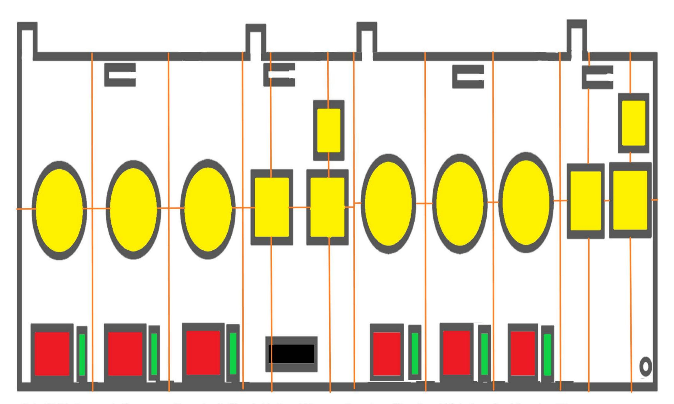
Note: All lids sit on a curb. The seams on the west end of the plant to the middle run up the curbs, and from the middle to the east end they stop at them. Entry to plant stariwells have a curb too that the seam runs through on the west end along with running through the pedestal for station service.
