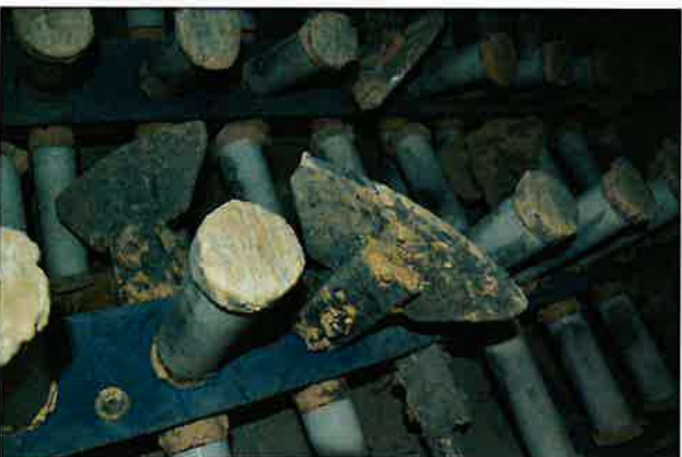
Figure 4.4 Interior of Pin & Paddle Mixer for Fugitive Dust Control (Preparation of Conditioned CCR)
